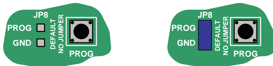
a) No Jumper: FPGA Operational (default)
