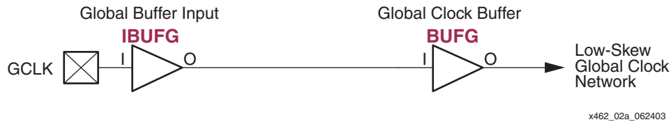
a. Global Buffer Inputs and Clock Buffers Drive a Low-Skew Global Network in the FPGA
